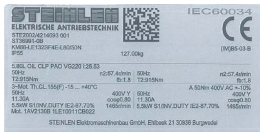
Figure 11-1 Example of a MOTOX rating plate
