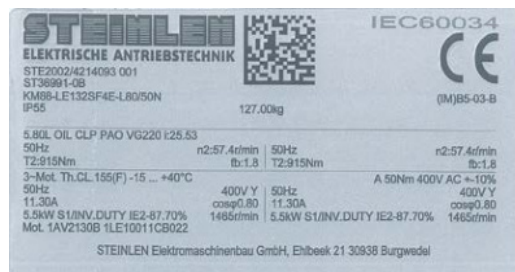
Figure 11-1 Example of a MOTOX rating plate
